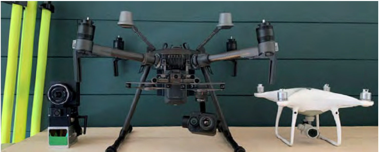
LiDAR/IR/HD Camera drone compared with normal 8 MP camera drone
