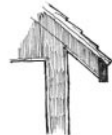
Cover rafter tails
