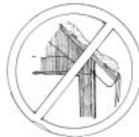
Unprotected rafter tails
