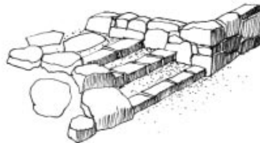
Steps and site wall Assemble natural, not overly refined materials
