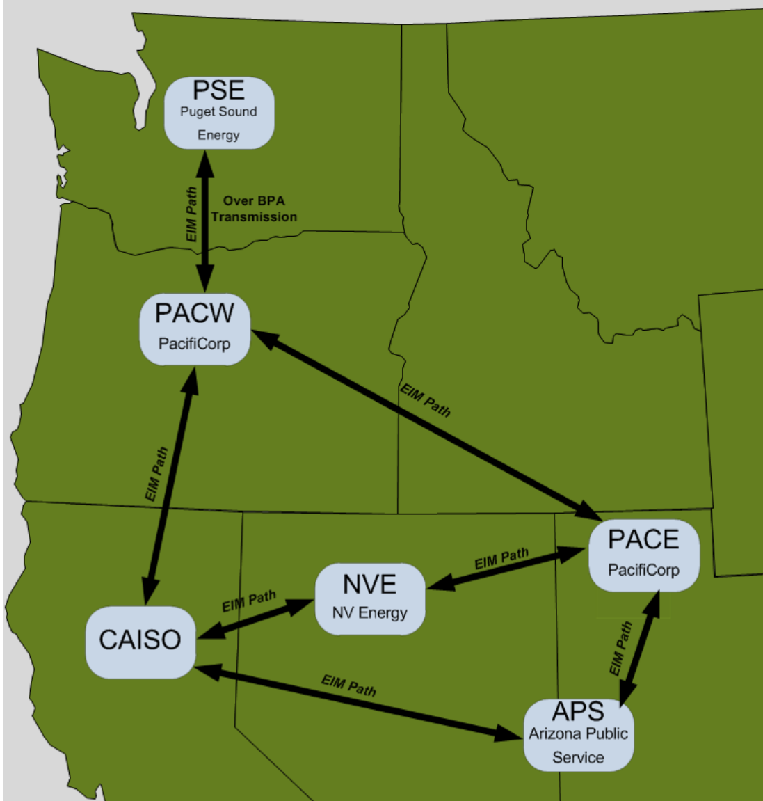
Figure I-4: Established EIM Transfer Paths as of October 2016
