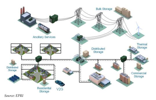
Figure L-1: Overview of Energy Storage Roles on the Electric Grid
