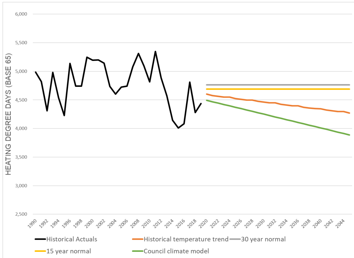
Figure 6-30: Annual Heating Degree Days (Base 65) for the Three Temperature Sensitivity Options Compared to 30-year Normal HDDs Used in the Base Demand Forecast
