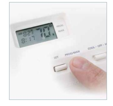
Connected thermostats control the HVAC system in order to maintain zone temperatures via the internet. Connected thermostats provide internet access to alerts, and monitoring and control from a remote location.
