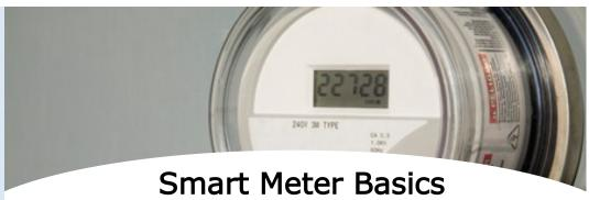
Smart meters communicate energy consumption data from your home to your electric company using brief low-level radio frequency (RF) transmission signals. These signals are safe and comparable to the level of RF signals that people are exposed to daily. For example, similar low levels of RF energy are emitted from cell phones and other popular
